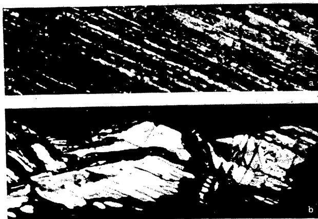
Fig. 5. Microphotographs of the rupture surfaces of single crystals deformed at -196^{\circ}\text{C} ( \times 70 ): a) sample 54; b) sample 69.
