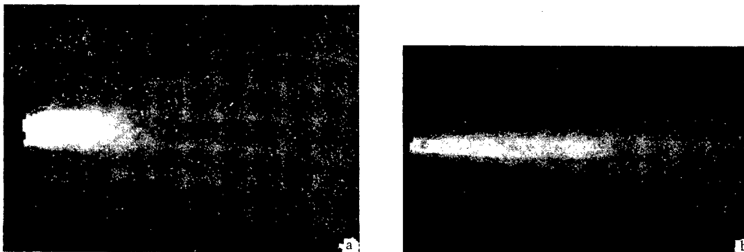
Fig. 1. Luminous regions in air excited by electron beams with energies of 1 (a) and 4 MeV (b).
