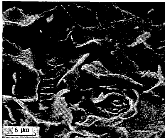
Fig. 2. Surface erosion of vanadium VTsU, irradiated at 770°K with He + ions with energy 100 keV up to a dose of 5 \cdot 10^{22} \text{ m}^{-2} .
