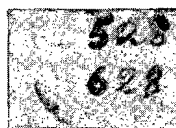
Fig. 1. Autoradiogram of a text consisting of figures, which was written with a methyl violet ink, after treatment with an \text{AgNO}_3 solution which was labeled with \text{Ag}^{110} . The original text was written a year and a half ago; a month before the investigation, the numbers 5 and 6 were added with the same ink.
