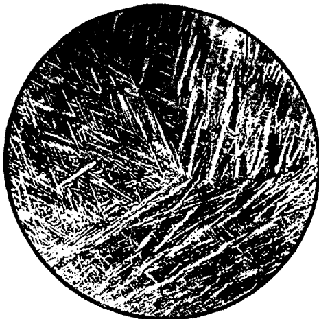
Fig. 6. Microstructure of the alloy from the first polythermal cross section containing 7% tantalum and niobium. Martensitic-like structure of the transformed \beta phase. Quenched from 1000^{\circ}C . ( \times 200 ).
