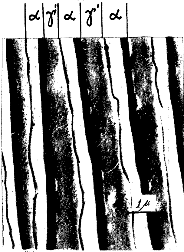
Fig. 3. Microstructure of uranium - 9 weight % molybdenum alloy after heating at 550° C for 1000 hours (x 17,000).
